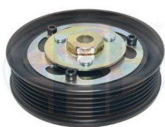
POLIE COMPRESSOR VAG 5Q0816803D 6P
