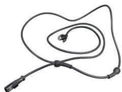
SENSOR ABS RENAULT TRS. DRT. 479506614R A4539055600
