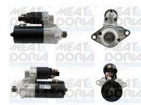
Item Number: 5010219 Component: 2 Teeth no: 10,11 Volt: 12 Flange Ø: 76 Connector ID: 30-50 Rotation: CW
