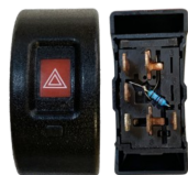
INTERRUPTOR EMERGENCIA OPEL 6F 24416080 =662035 =23602
